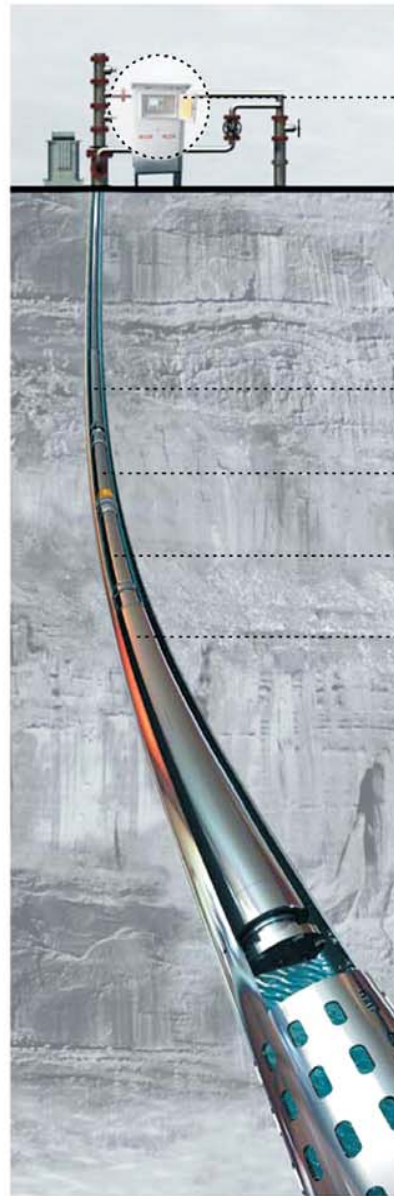
Submersible centrifugal pump (Formation fluid lift)
